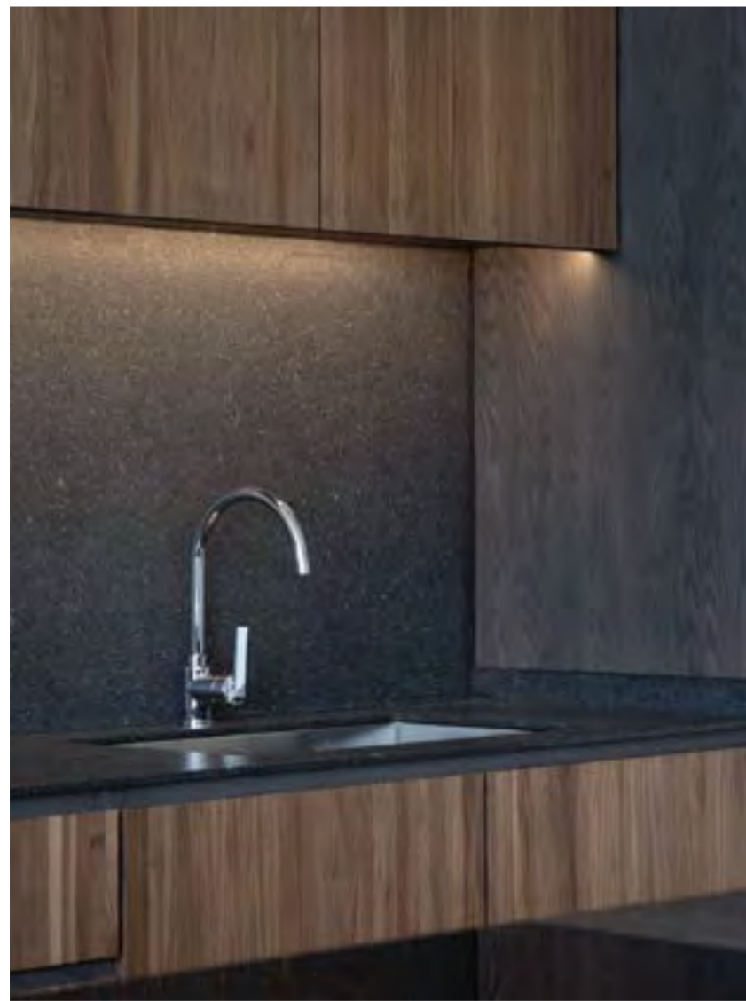
Above: A close-up of hidden 3000K LED strip lights under the hanging unit with walnut wood doors in soft natural walnut wood finish.
