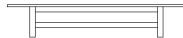
PIER bench w 2000 x d 380 x h 440 w 1800 x d 380 x h 440 w 1600 x d 380 x h 440
