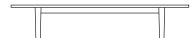
MULTO bench w 2400 x d 375 x h 440 w 2000 x d 375 x h 440 w 1800 x d 375 x h 440
